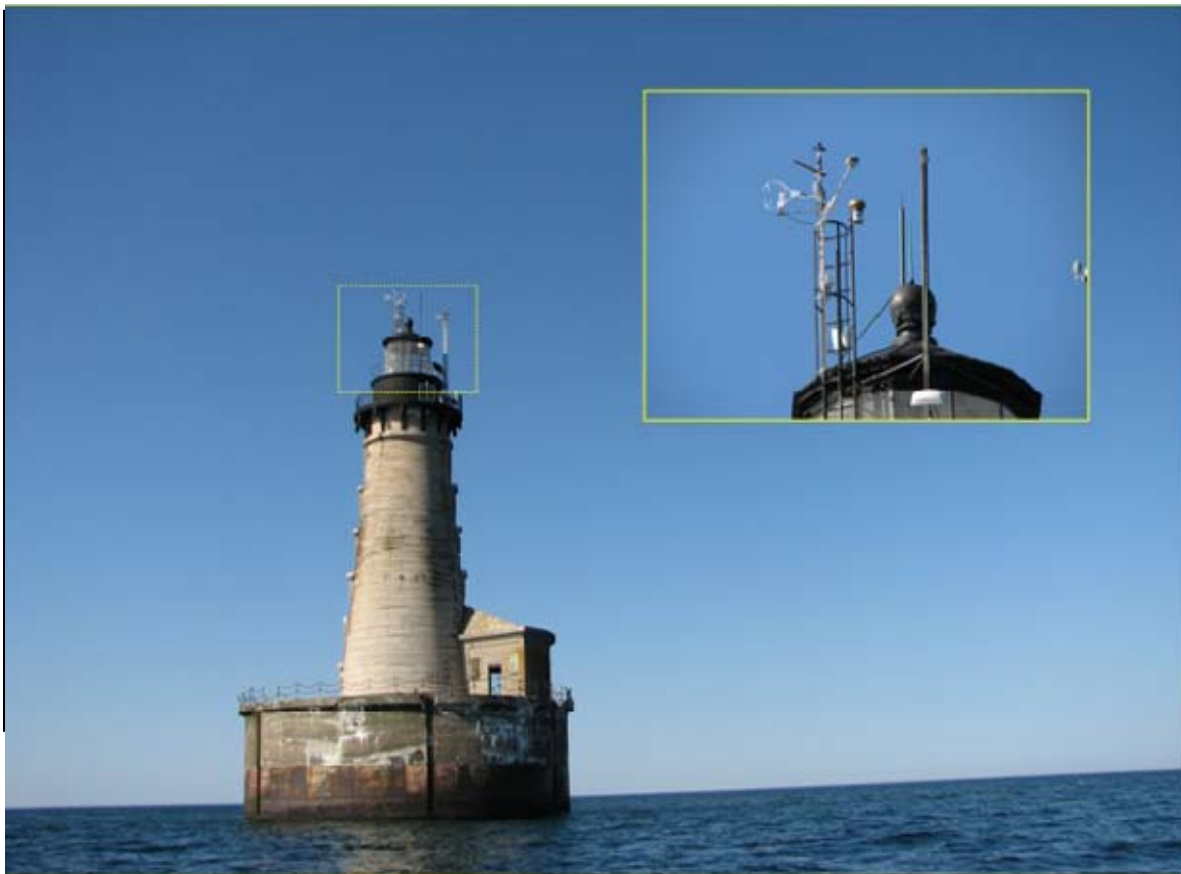
Stannard Rock Lighthouse with inset of eddy covariance instrumentation tower Photos courtesy of Chris Spence and Newell Hedstrom
